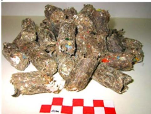
**Figure 4 Pellets produced from waste after biological drying**
